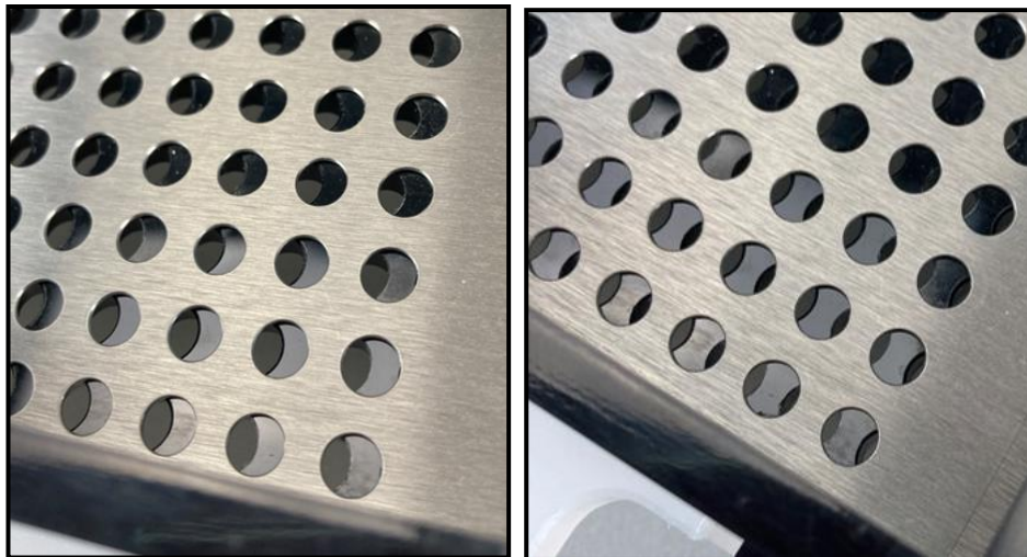
Incorrect (left) and correct (right) sliding plate position relative to top plate.
