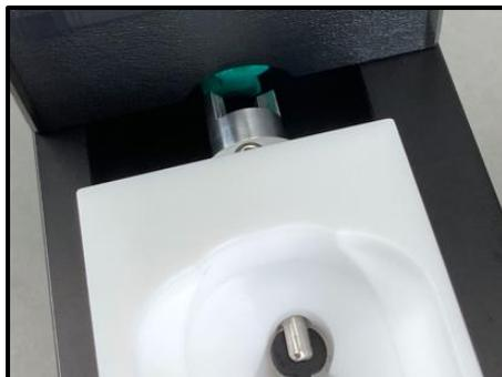
**Figure 3. Aligning aluminum jaws of Reservoir coupler with green motor coupler.**
