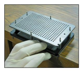
9. Screw hex nuts onto the screws. Do not tighten down completely until all pins are in.
