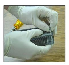
4. Place bottom plate so that counter-sunk screw holes are facing down. Place BGP onto the bottom plate so that the guide pins go through the two notches.
