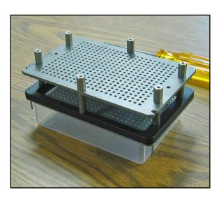
10. Place pins carefully back into the replicator. Make sure all pins float and then tighten down the hex nuts completely.
