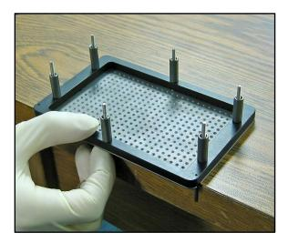
8. Place middle plate on the screws so that the counter-sunk pin holes are facing up.
