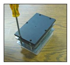
2. Remove pins into vials. Be careful not to bend the pins.
