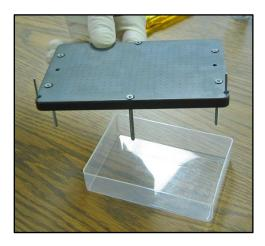
6. Flip replicator over and position it so that it's on the edge of a table. One side screw will need to be held in or else it will fall out.
