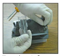
3. Unscrew hex nuts. Remove screws and spacers from replicator.
