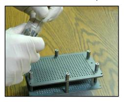
3. Unscrew hex nuts while ensuring that screw heads on bottom do not turn. Remove screws and spacers from replicator and you will have only the bottom float plate remaining.
