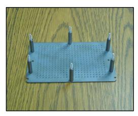
6. Put top float plate on spacers with pin holes counter-sunk up (screw holes are not counter-sunk in either direction).
