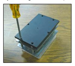
2. Remove pins to vials. Be careful not to bend the pins.
