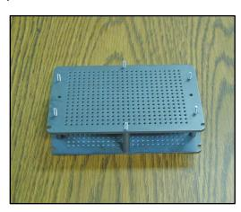
7. Place some Loctite (if available) on each screw and then screw a hex nut onto each screw.
