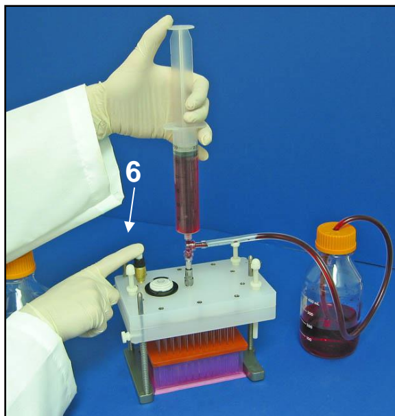
Figure 4. Bleeding Air from Manifold by Filling with Liquid using Syringe or Bottle Top Dispenser.
