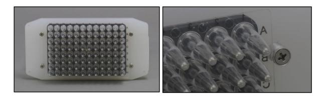
It is important that there is not a gap between the magnetic pins and the end of the Cover Plate's pointed wells. V&P's Cover Plate VP 407AM-N1-PCR is designed to make sure there is no gap.
