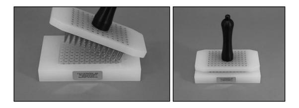
The short edges of the Cover Plate must be held in place by all 4 of the clips for proper positioning.
