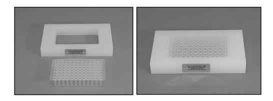
The VP 407AM-N1 is then positioned over the Cover Plate and firmly lowered until it clicks into place.
