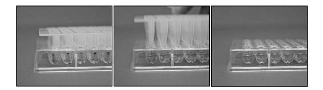
**Optional Magnetic Separation Block to use with the VP 407AM-N1:** The destination microplate with the detached Cover Plate can then be placed on a magnetic separation block, such as VP 771RWAM-1 (below left) to ensure all the beads are removed from the Cover Plate before discarding.
