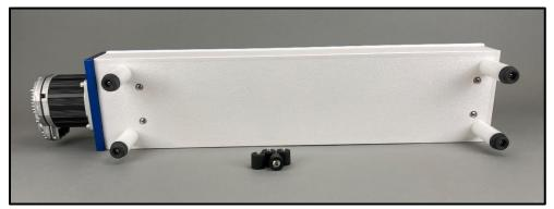
To change back to the short rubber feet, unscrew the extensions by hand. Note that sometimes the set screw will stay the hole in the stirrer instead of the extension. Remove the set screw from the stirrer with 1/8<sup>th</sup> Allen wrench and replace into the extension for safe keeping. Take care to not cross-thread the screw in the threads of the extension.
