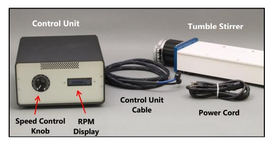
Attach the Control Unit Cable (thick black cable with two plugs) to the Tumble Stirrer using the two connection ports found on the side of the motor. The smaller plug goes into the bottom port, while the large plug with blue cable into the top one. Each plug has a release tab the needs to be on the outside when plugged in. Attach the Power Cord to the Power Connection Port on the back of the Control Unit (see the photos below).
