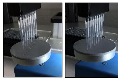
To align pipet tips to inside of SpinVessel® tube, use the registration disc. Place disc on top of the drive base, not the tube. Lower the tips until they just touch the disc. Align tips to the holes.
