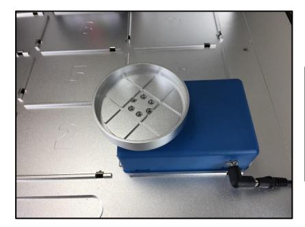
Place SpinVessel® motor unit in desired location, either on an automated liquid handler or on a benchtop.
