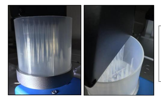
With the SpinVessel® tube in the drive base, check the tip alignment relative to the projections.
