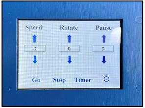
Upon power up the startup screen shows the following control features: **Speed:** 0-100% (this does not reflect RPM) **Rotate:** Number of rotations between pauses **Pause:** Pause time in milliseconds the device pauses between rotations
