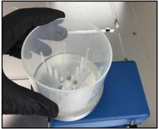
Insert the SpinVessel® tube VP 830SV-300FB into the SpinVessel® drive base.
