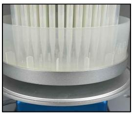
With the SpinVessel® tube in the drive base, check the tip alignment relative to the projections.
