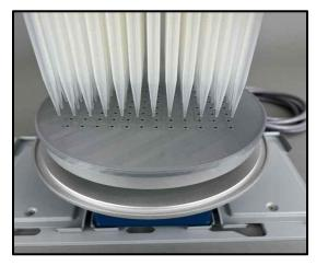
To align pipet tips to inside of SpinVessel® tube, use the registration disc. Place disc on top of the drive base, not the tube. Lower the pipet tips until they just touch the disc. Align robot tips to the holes. This registers the pipet head to the SpinVessel® and prevents the pipet tips from hitting the SpinVessel projections.
