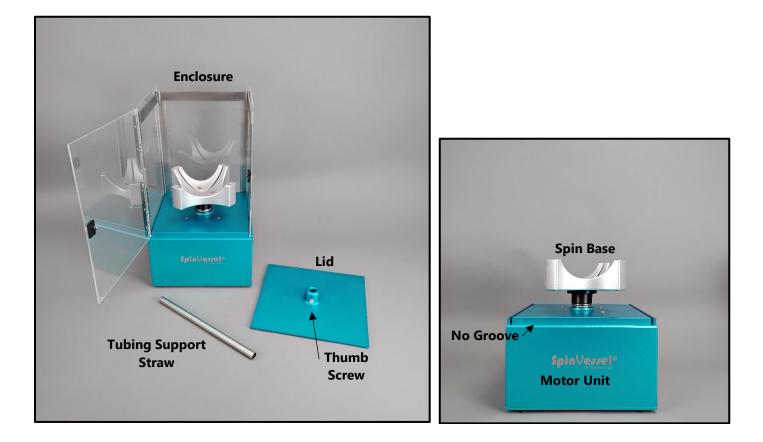
2. Place the Lid on top of the Enclosure also making sure it is resting firmly in the groove on the underside of the lid. In addition, position the one side of the lid that does not have a groove above the door of the Enclosure.
