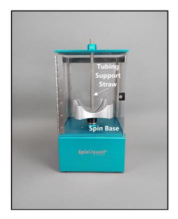
6. Insert the SpinVessel® VP 830SV-6L into the SpinVessel® Spin Base. Ensure that the tabs on the outside of the SpinVessel® are seated flat and registered to the slots in the aluminum Spin Base.
