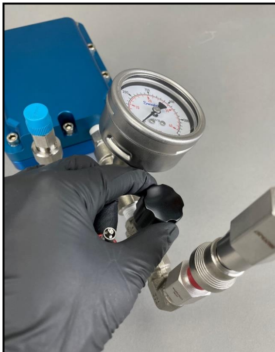
Figure 11. Inlet Valve opened.
