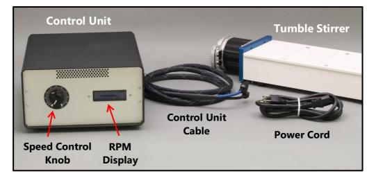
Attach the Control Unit Cable (thick black cable with two plugs) to the Tumble Stirrer using the two connection ports found on the side of the motor. The smaller plug goes into the bottom port, while the large plug with blue cable into the top one. Each plug has a release tab the needs to be on the outside when plugged in (see below).
