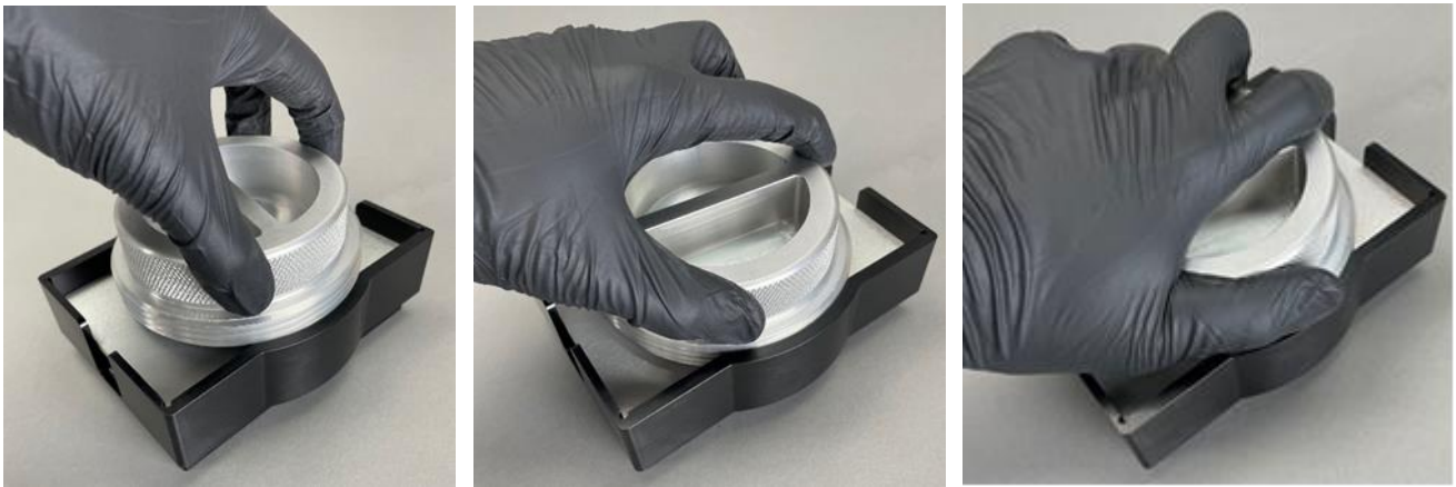
Figure 7. Views of tightening puck being aligned, screwed down until engaging the aluminum lid and final tightening
