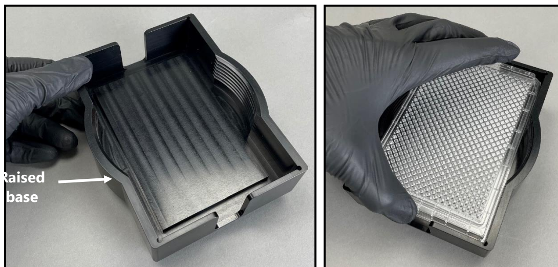
Figure 3. (a) Microplate block: smooth, flat and debris-free (b) Using finger guides to lower microplate into base
