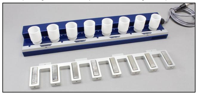
5. Lift the Magnet bar so that it is vertical and insert the tabs into the trapezoidal holes in the Support Rail. Secure with the final two screws
