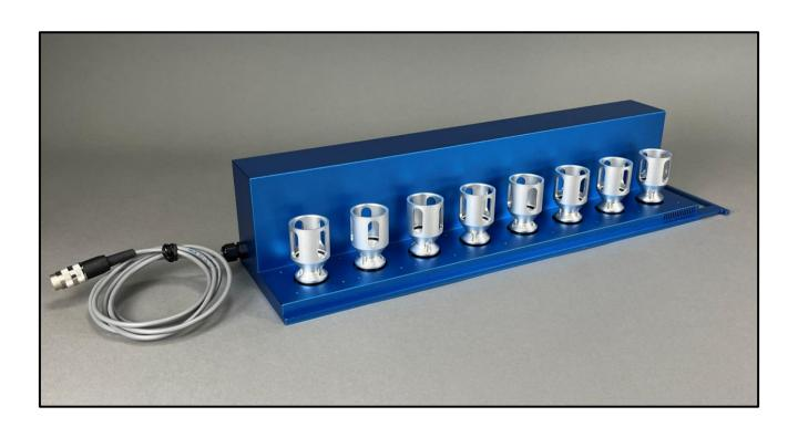
VP 418SVG-1X8HS50-CC SpinVessel® GEARED MOTOR SYSTEM, for 8 x 25mL/50mL Conical Bottom SpinVessel® (in a 1x8 array), made for Hamilton Star and Vantage Liquid Handlers, Direct Drive Stepper Motor, Aluminum Enclosure, Computer Controlled via ASCII Commands, API and Drivers on USB, 100/240 Volts, 50/60 Hz, CE Compliant
