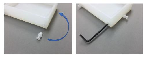
Use elbow hose barb fittings for tubing attachment to the side ports and straight hose barb fittings for tubing attachment to the front ports.
