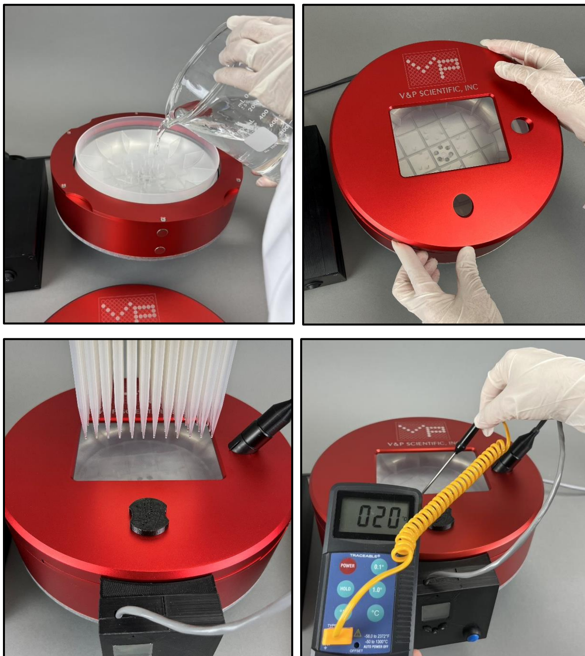
Figure 8. Pouring pre-heated solution in SpinVessel in the Circle Heater. Replacing the lid in the proper orientation for use with 96 channel pipet head. Independent check of solution temperature.
