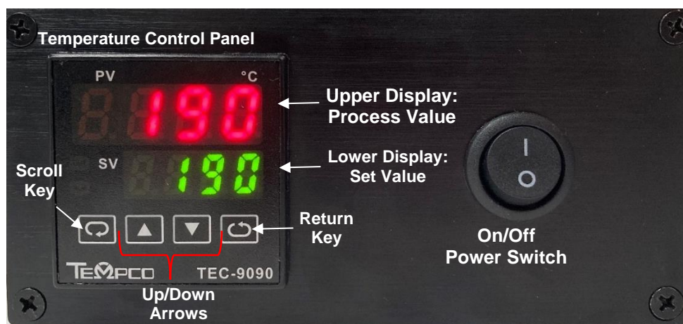
Figure 7. Front View of Temperature Controller for the Circle Heater.
