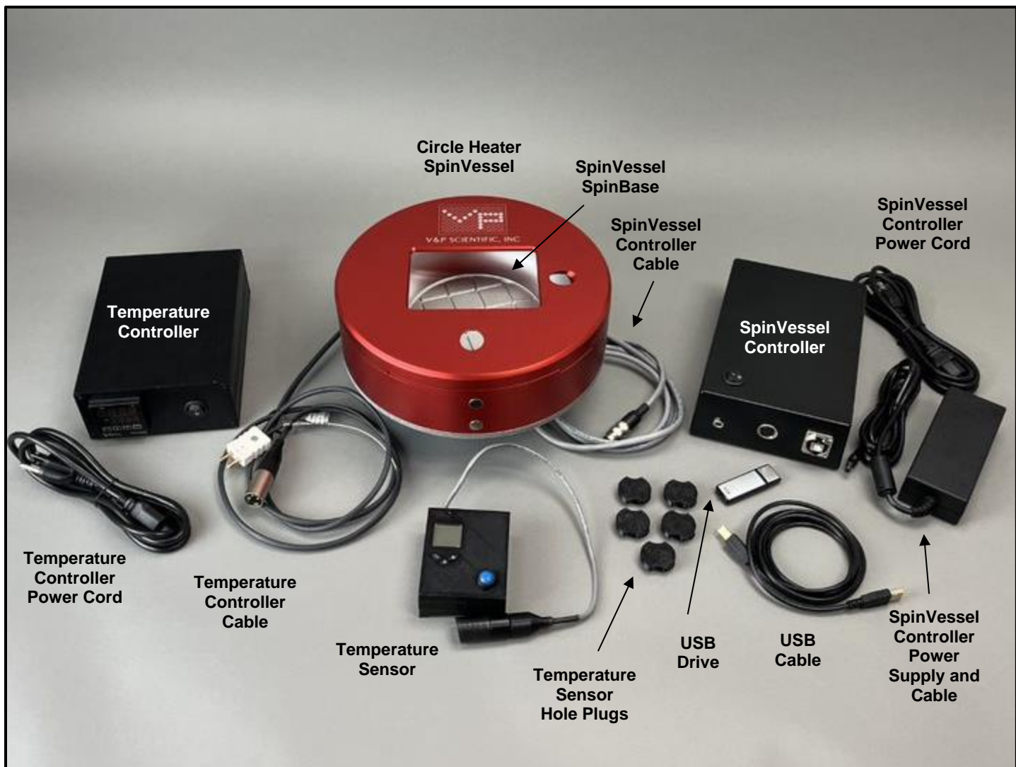
Figure 2. Parts of the Circle Heater SpinVessel® VP 418SV2-H-1LFB-CC.
