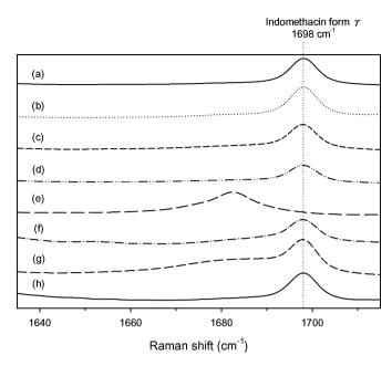
**Fig. 3.** Raman spectra of indomethacin and aromatic acids slurried in the well plate after 7 days. Aromatic acids were hippuric acid (a); benzoic acid (b); gentisic acid (c); salicylic acid (d); D/L-mandelic acid (e); 1-hydroxy-2-naphthoic acid (f); 2,5-dihydroxybenzoic acid (g); and p-hydroxybenzoic acid (h).
