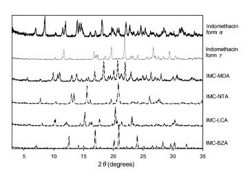
**Fig. 7.** PXRD patterns of scaled-up indomethacin, cocrystal former, and indomethacin cocrystals.
