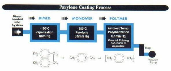
Parylene is not produced or sold as a polymer. It is not practical to melt, extrude, mold or calender as with thermoplastics. Nor can it be applied from solvent systems. Actually, many of the advantages found in parylene coatings, unlike epoxies, urethanes or silicones are a direct result of the coating deposition process.
